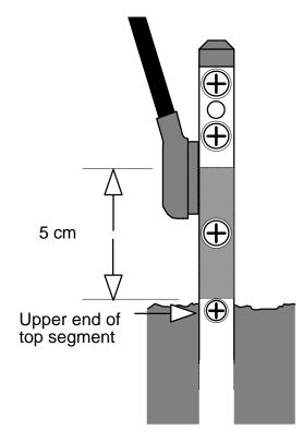
To obtain reliable moisture readings from the top segment of a profiling probe it is important to ensure that the probe is inserted to the proper depth. The soil/air boundary should be level with the upper screw of the top segment. There are two types of screws along the side of the probe. The sizes of these screw are 10-24 (large) and 6-32 (small). On all standard probes the uppermost 6-32 screw is the upper diode screw of the top segment.
