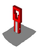
Attach the coupling link to the pilot rod using the hardened steel dowel pin provided. Insure that only the correct hardened steel dowel pins are used with the coupling link. Undersized dowel pins may eventually enlarge the holes in the pilot rod and probes, and underrated dowel pins may break under load. *DO NOT use shear pins.* Replacement pins are available from ESI.
