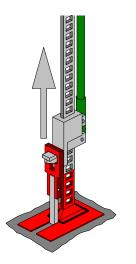
With the coupling link attached to the pilot rod, slip the large opening over the jack head lifting nose and insure that the center of lift will be vertical and parallel to the jack standard.
